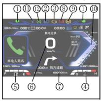
The instrument panel of this model can be set to daytime interface mode or night interface mode or automatic mode (the instrument panel automatically switches to daytime or night interface when it senses ambient light conditions).
